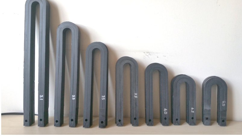
Figure 4-5: Set of springs with different rotational stiffness values. The longer the spring, the more compliant it is.
