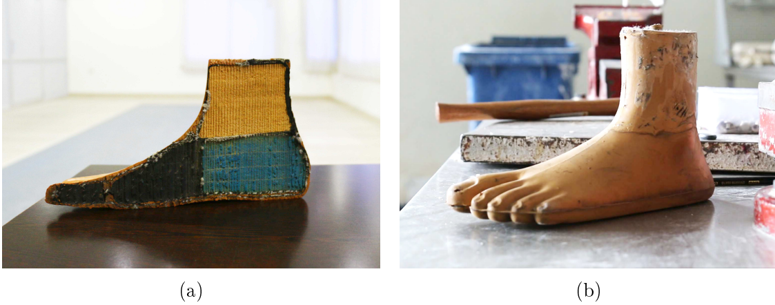
Figure 1-1: Photographs of the Jaipur Foot. (a) Cross-section view, with the wooden block at the ankle and the two rubber blocs covered by an aesthetic vulcanized rubber layer (b) Full view of the foot.
