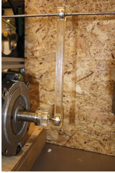
Figure 10: Image of the crank shaft system setup, with ajustable crankpins to set different forcing amplitudes. The square frame of the soap film is mounted on vertical rail guides actuated by the connecting rod.
